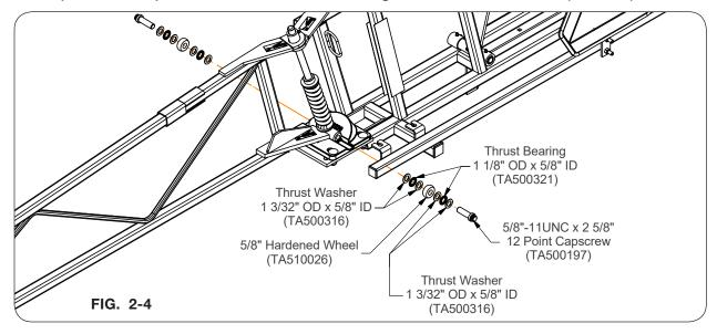
4. Tighten wheel capscrews so it turns tightly (FIG. 2-4). Wheel should not spin freely.
